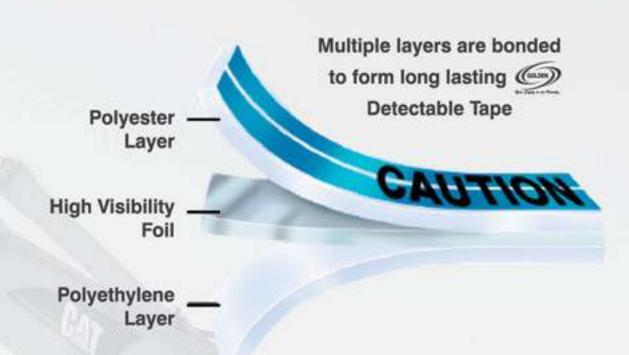
"GOLDEN" Brand Aluminum strip detectable tape is a strip of detectable aluminum foil totally encapsulated between a polythene base layer and a printed polythene protective covering with a 10 - 50 mm wide aluminum strip and is not less than 10 - 12 micron thick. When buried, the Alu.strip has contact with the earth for its entire length maximizing the potential for inductive location. The aluminum strip detectable tape is mainly used for marking of non-metallic underground pipes and cables.
